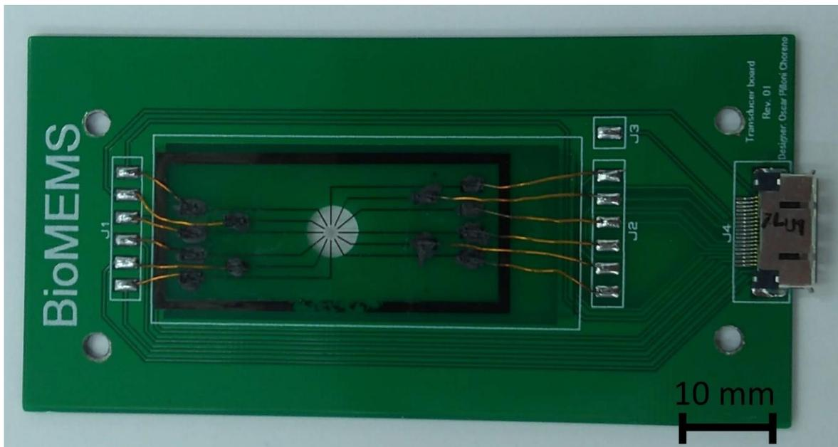
Fig. 28: Photograph of the complete electronics interface board with C-MEMS microelectrodes connected to the PCB.
