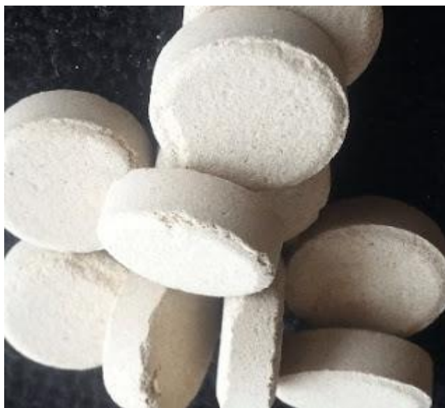
Figura 7: Astillado/ “Chipping” de tabletas (Choudhary, Ankur (Pharmaceutical Guidelines);, 2018).
