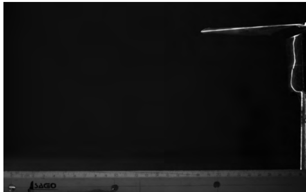
Figure 4.5: Calibration used to measure the distance from the rotor to any given point in the image. In this picture, one can see part of the helicopter.
