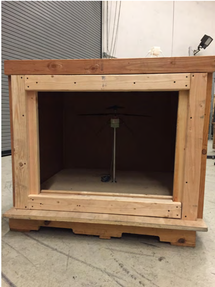
Figure 4.1: Test cell box. The fuselage inside the box is the half-scale model.
