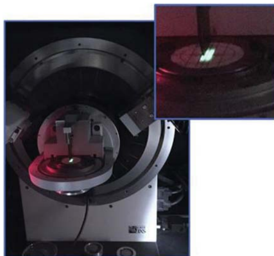
Fig. 2 Experimental measure of spot size length along the diffraction plane at different angles
