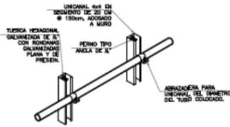
**DETALLE A SOPORTERIA DE UNICANAL SIN ESCALA**
