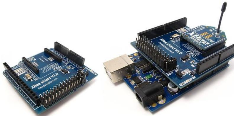
Figura 6. XBee Shield V1.1
