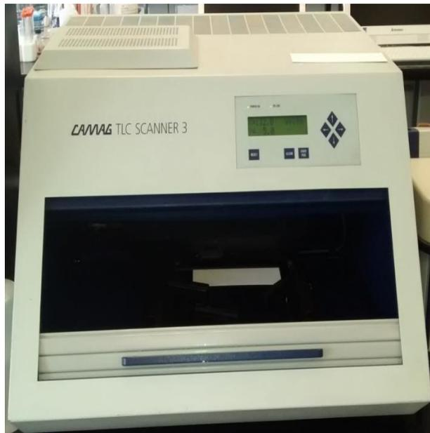
Figura 37 Detector de HPTLC, TLC Scanner 3
