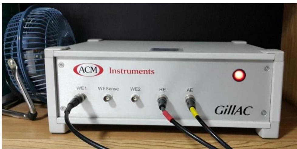
*Figura 27 Potenciostato Gill ACM Instruments*
