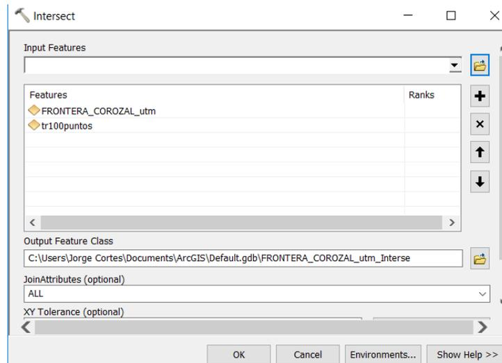
Figura 4.10 Herramienta geoprocessing/Intersect de (ArcGISV10.4®)
