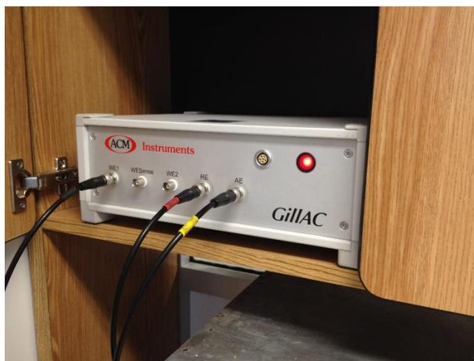
Figura 3.12. Potenciostato-Ganvanostato ACM Instruments Gill AC
