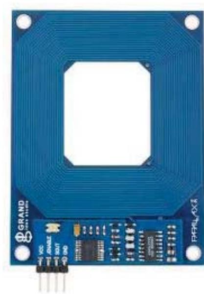
Fig. 149 | Parallax RFID Card Reader
