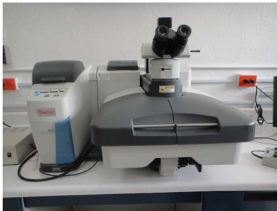
*Figura 57. Microscopio  $\mu$ -Raman.*
