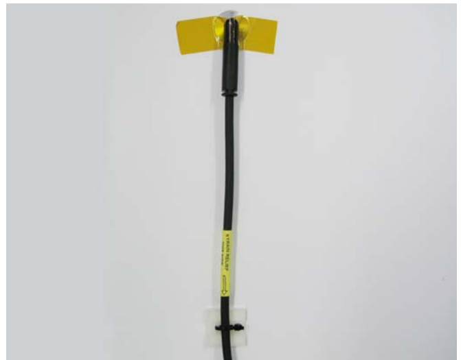
The 110PV is mounted to the measurement surface via Kapton tape.
