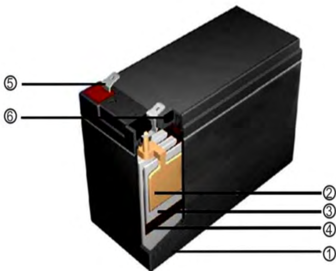
Fig. 51: 1. Container/Cover: Made of UL94HB and LU 94V-0 ABS Plastic 2. Negative Plates: Use the special PbCa alloy grids, optimize the recombination efficiency and less gassing. 3. Separator: Import high quality AGM separator. 4. Positive Plates: PbCa grids minimize corrosion and prolong life. 5. Terminal post: Cooper material with maximum conductivity, rapidly.
