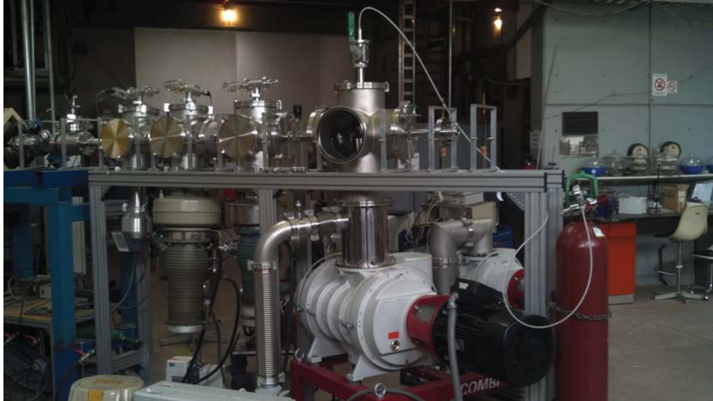
Figure 4.8: Finished line - A photograph showing the finished beamline for the supersonic gas jet target.
