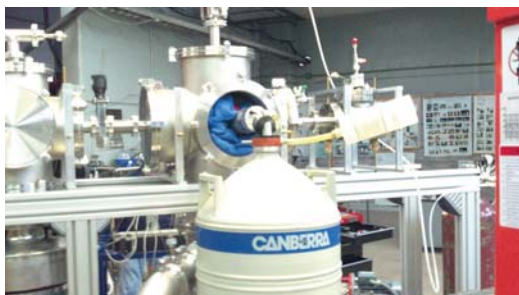
Figure 4.23: Germanium Detector - The experimental array with the germanium detector in place.
