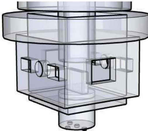
Figure 4.2: Square chamber - A 3D sketch of the scattering chamber as a box. It has X-ray view so the inside is shown.
