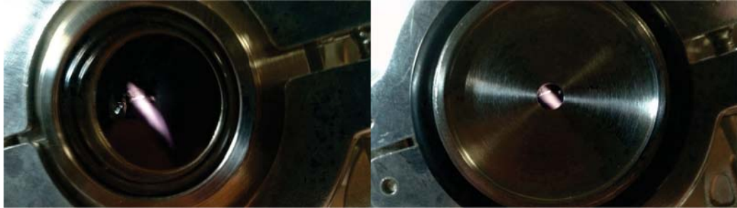
Figure 4.18: The Beam - Shows how part of how the alignment was made with the beam hitting the view port inside the differential pumping chambers. Left shows the beam, right shows the beam through a 5mm diameter hole.
