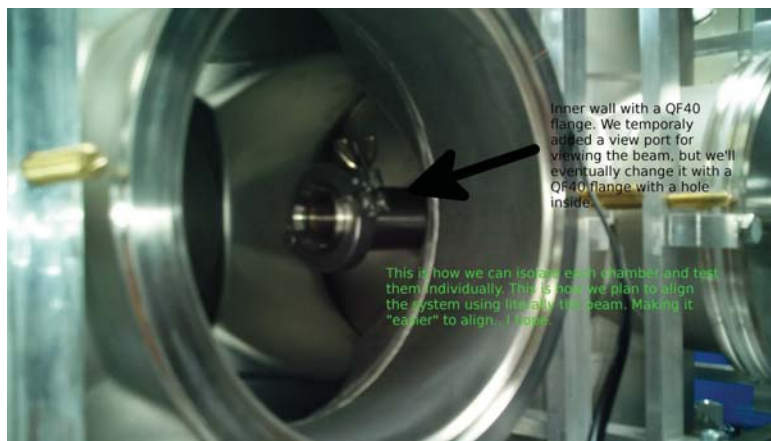
Figure 4.17: Inner Wall - A wall with a QF40 adapter was placed in between the differential pumping chambers. For placing QF40 blank flanges with small apertures.
