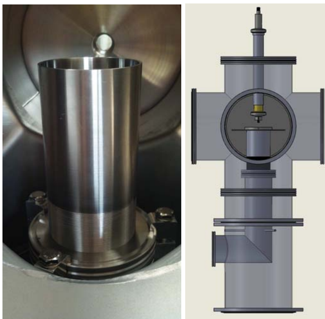
Figure 4.13: The catcher - Shows the adjustable height jet catcher and the scattering chamber.
