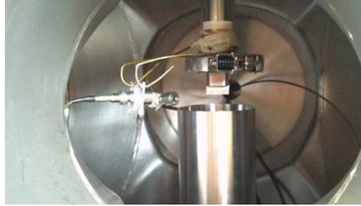
Figure 4.20: Inside The Scattering Chamber - Shows the nozzle , the catcher, the detectors and their improvised holders.
