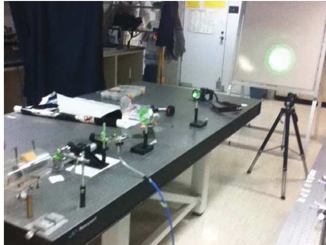
Figure 4.26: The Schlieren Physical Setup - Optical array to visualize the jet.
