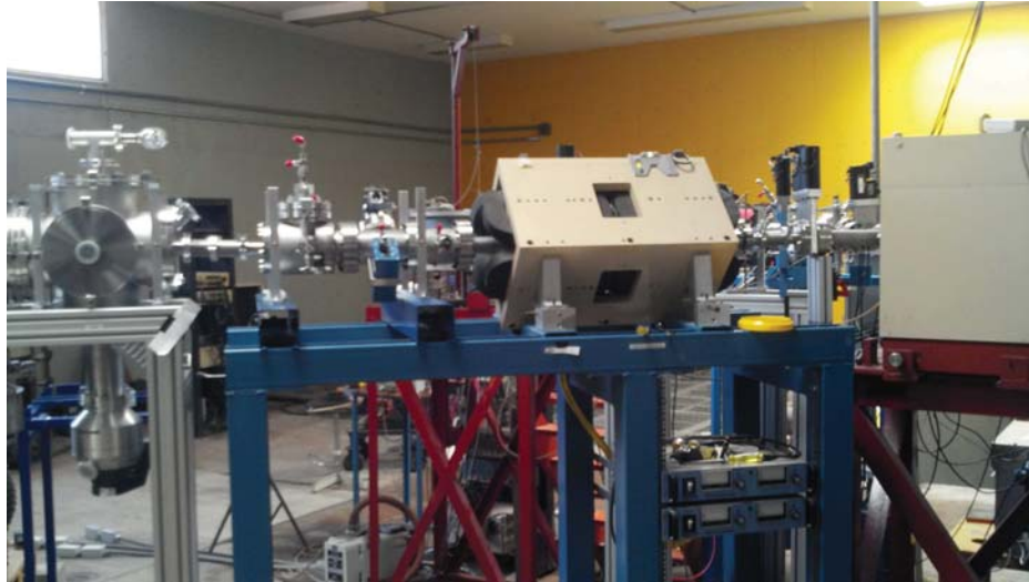
Figure 4.10: The Train - Right after the beam selector magnet and before the differential pumping system. It consists on a quadrupole magnet, slits, a beam profile monitor and a Faraday cup.
