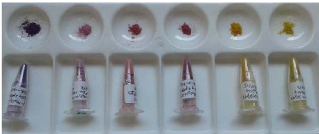
Fig. 4. Hybrid pigments based on chromophores stabilised onto gamma-alumina, from left to right: carminic acid, betacyanin extract, alizarin, purpurin, curcumin and fluorescein.
