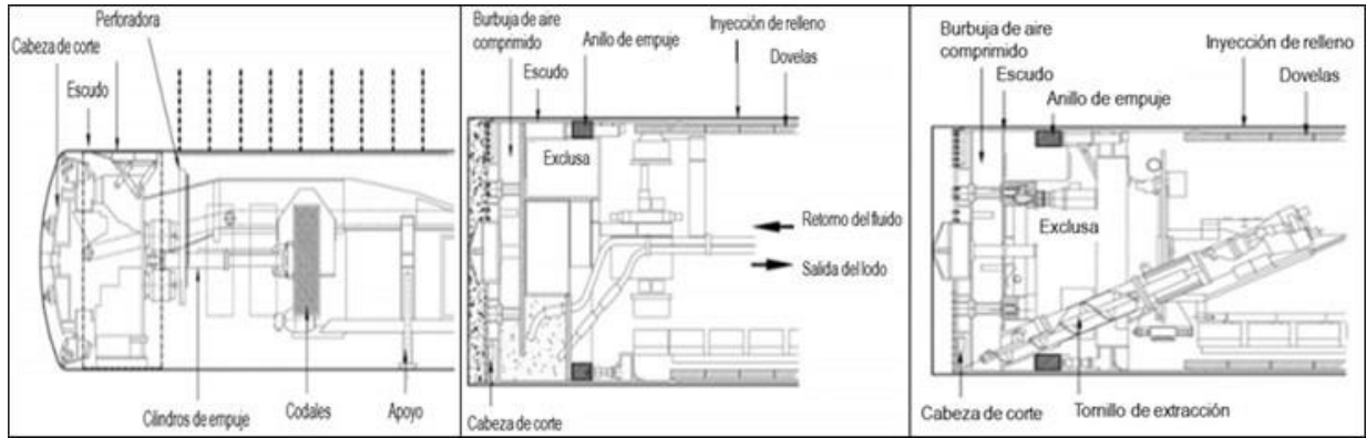
Tunnel Boring Machine.
