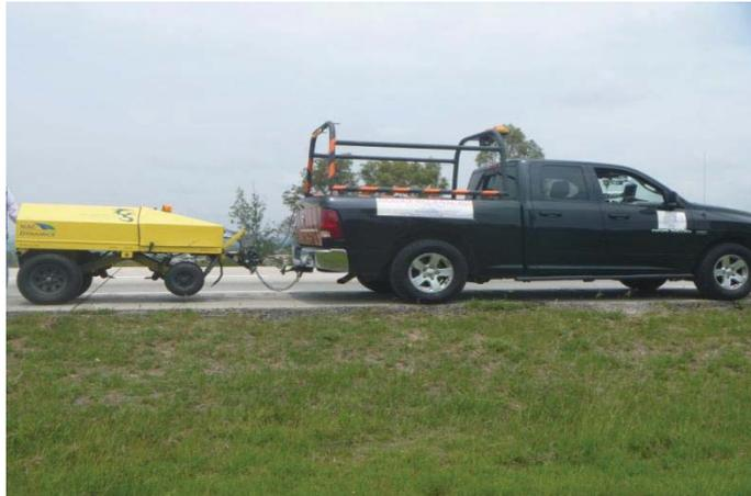
Figura 6.6. Mu-Meter, tipo DFT (Dynamic Friction Tester), marca NAC Dynamics LLC.
