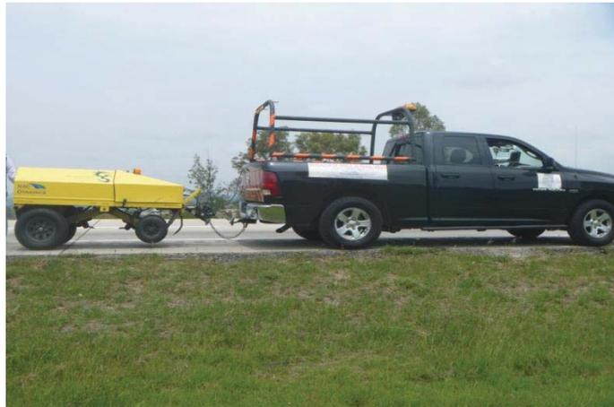
Figura 3.36. Mu-Meter, tipo DFT (Dynamic Friction Tester), marca NAC Dynamics LLC.
