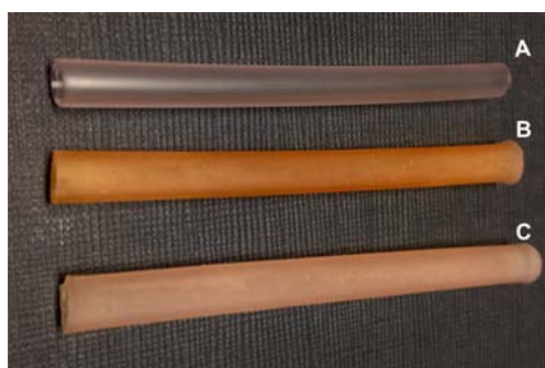
Figure 5.11: Color differences between (A) PVC, (B) PVC- g -PEGMA(15%), and (C) [PVC- g -AAc(12%)]- g -PEGMA(19%)
