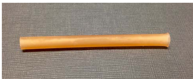
Figure 5.5: PVC-g-PEGMA(25%) catheter grafted using a 16% (v/v) aqueous PEGMA solution, 60 kGy dose, and T = 70\text{ }^{\circ}\text{C} .
