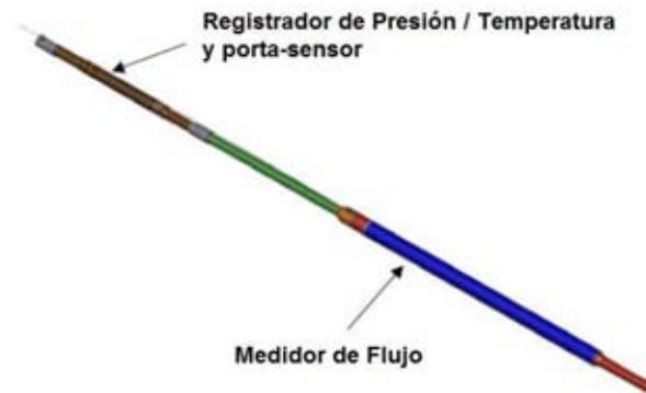
Fig. III.26: Sistema de medición de flujo de fibra óptica (Fuente: T.K. Kragas, F.X. Bostick, and C. Mayeu, paper SPE 77655 presented at the SPE Annual Technical Conference and Exhibition held in San Antonio Texas, September 29-October2, 2002)
