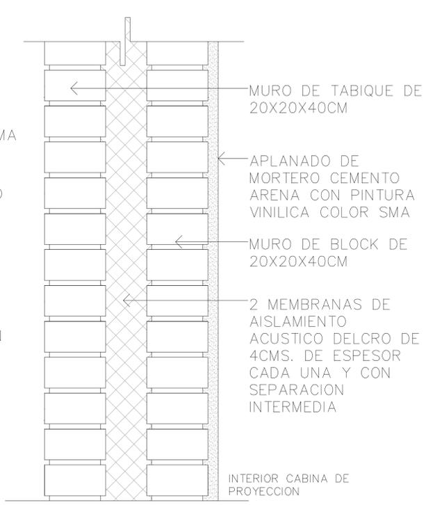
D-3 MURO DOBLE CON AISLANTE
