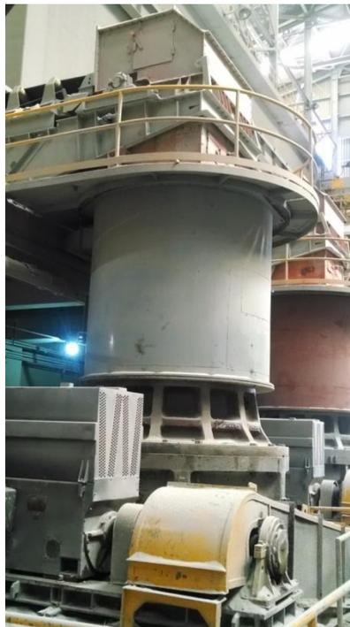
FIG. 2.65 Quebradora terciaria *Allis Chalmers/Kobe Steel* 3" x 84".
