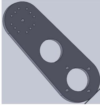
*Figure 11. Primary link of the Spatial Parallel Manipulator*
