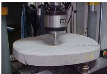
Figura 1.15 Ensayo de panel circular (ASTM C1550)
