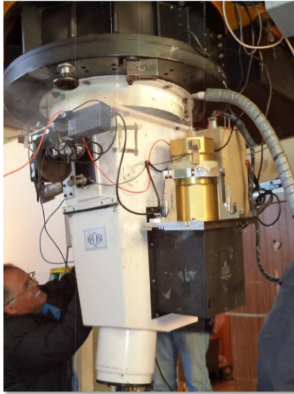
Figure 8. Mechanism integrated in the 2.1 m telescope.
