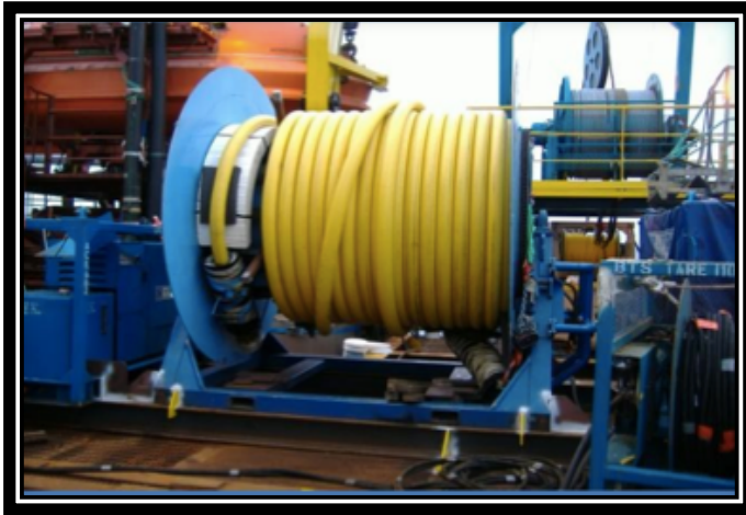
Figura 1.12. Riser flexible. (bunessanprojectengineering.com; 2010)
