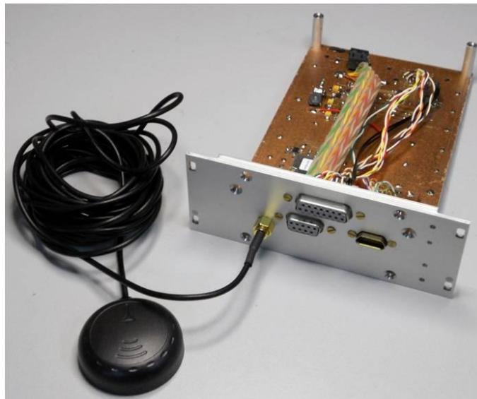
Figure43. GPSR mounted and tested [46].
