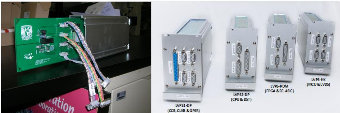
Figure77. LVPS-HK mechanical assembly (at left), and LVPS modules structures (at right).
