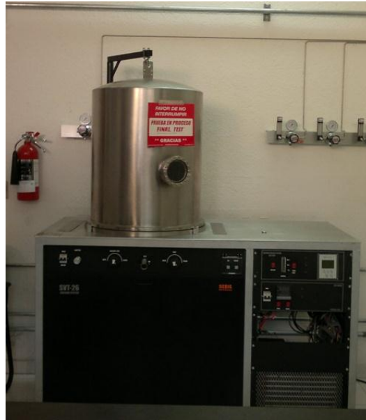
Figure81. Custom-made vacuum chamber.
