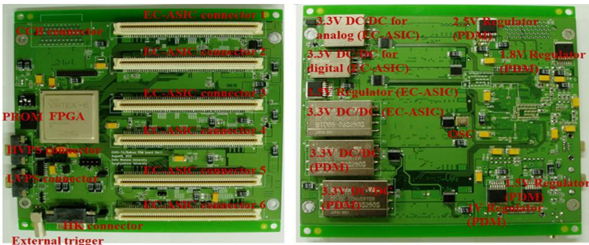
Figure37. PDM board prototype, top-layer at left, and Bottom-layer at right [44].
