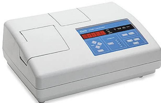
[Imagen 2. Turbidímetro, (camlab.co.uk)]
