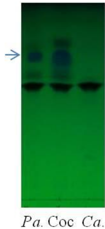
Supplementary Figure S5. TLC assay for PQS (arrow). TLC plate run with supernatant extracts from P. aeruginosa ( Pa. ), cocultures ( Coc. ) and C. albicans ( Ca. ). TLC was run using a mixture of dichloromethane:methanol (95:5) as the mobile phase and visualized using a UV transilluminator at 312 nm, and photographs were obtained at this point.
