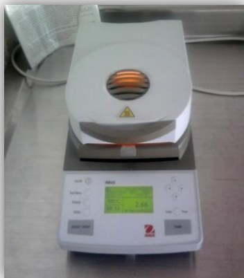
Figura 8. Termobalanza digital OHAUS MB-45.
