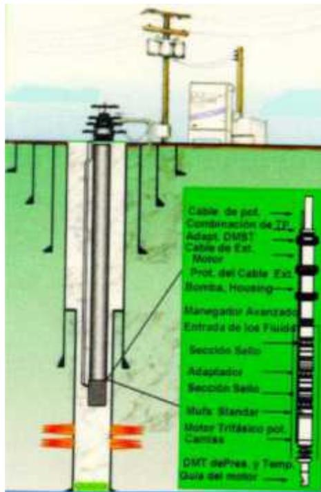
Figura 2.12 Bombeo electrosumergible
