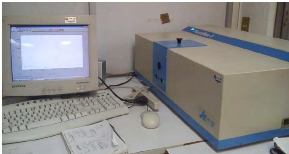
**Figura 4.5** Espectrofluorimetro FluoroMax-3.
