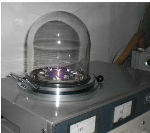
Figura 41. Ion-sputter JEOL modelo JFC-1100E.
