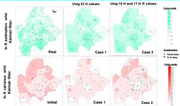
Figure 3. Up. Plot of the ln K realization (left), the ln K estimation Case 1 (center) and Case 2 (right). Down. Plot of the initial variance (left), final variance Case 1 (center) and Case 2 (right).
