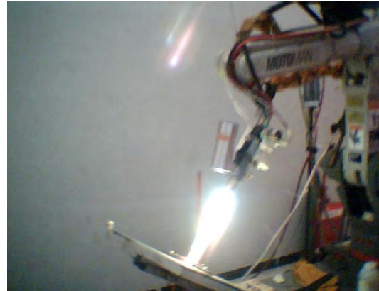
Fig 14: Image of the automated combustion powder thermal spraying process.(ACPTSP) operating.
