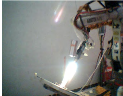
Fig 13: Image of the automated combustion powder thermal spraying process.(ACPTSP) operating.
