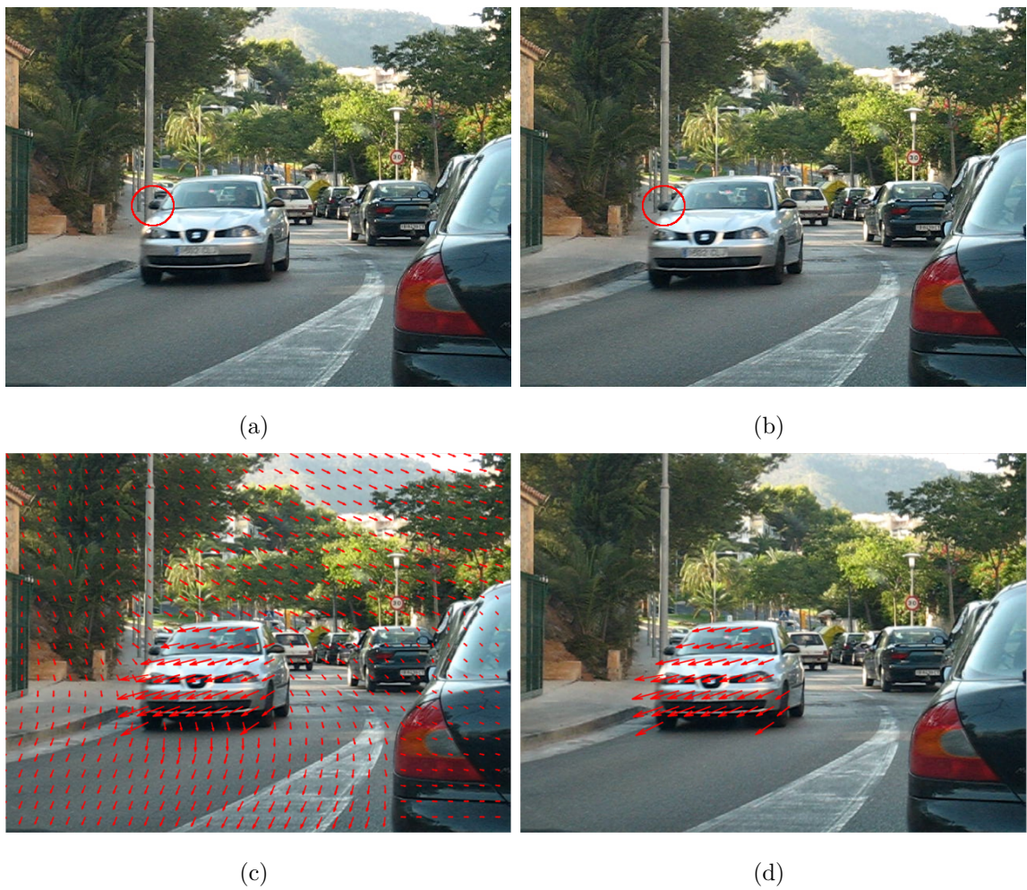
Figure 3.2: Optical flow representation in a sequence of images. (a) Frame 43 of the Cameramotion sequence. (b) Frame 44 of the Cameramotion sequence. (c) Optical flow. (d) Segmentation of the car using displacement vectors.
