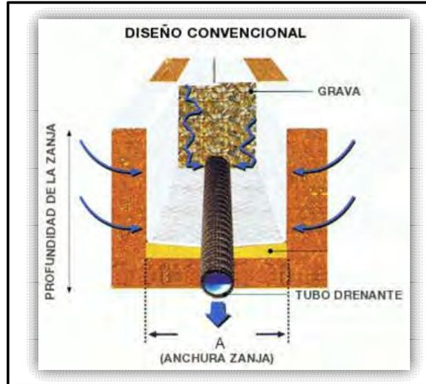
FIG. 1 DIAGRAMA DE UN DREN CIEGO O DREN FRANCÉS
