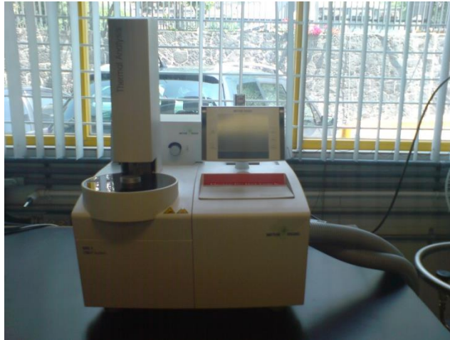
Figura A.6.1 DSC 1/700/1694 METTLER TOLEDO.
