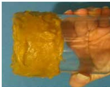
**Fig. 8** Finished molded biopolymer.
