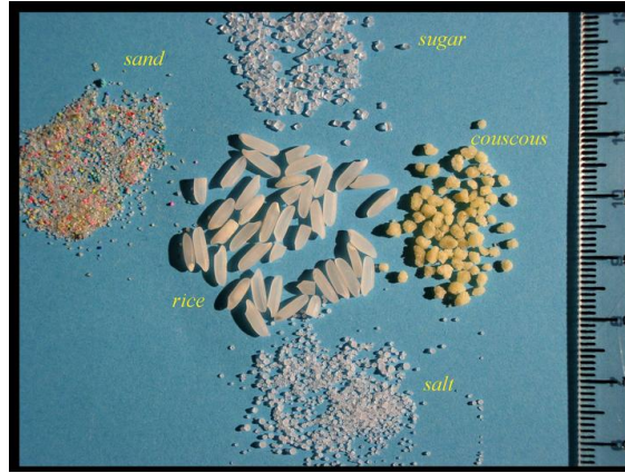
Figura 2.1: Example of materials used for the collapse of granular columns. Figure from [30].
