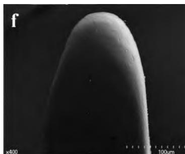
**Fig. 4-11. Microfotografía de la punta no cortante de RaCe. Tomada de Oh SR, Chang SW, Lee Y, Gu Y, Son WJ, Lee W, et al. A comparison of nickel-titanium rotary instruments manufactured using different methods and cross-sectional areas: ability to resist cyclic fatigue. Oral Surg Oral Med Oral Pathol Oral Radiol Endod. 2010;109(4):622-8.**
