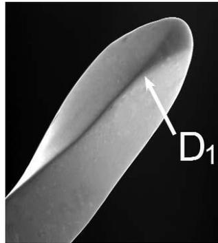
Fig. 2-5. Punta no cortante del instrumento EndoSequence. Tomada de Kurtzman GM. Simplifying Endodontics with EndoSequence Rotary Instrumentation. J Calif Dent Assoc. 2007; 35(9): 625-8
