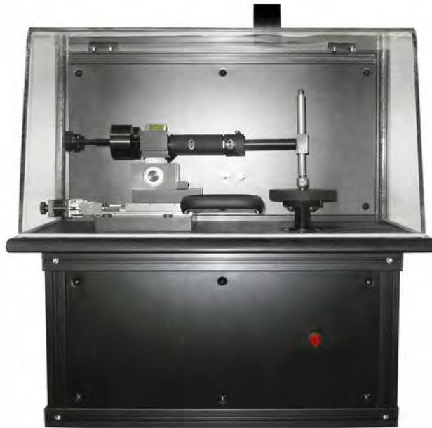
Figura 3.7 Tribómetros pin-on-disc NANOVEA (Nanovea company-Irvine-USA)
