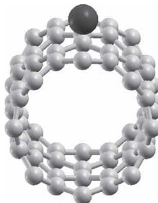
Figure 1 Optimized configuration using LDA of a single-walled carbon nanotube with one adsorbed Li atom with coverage C_{64}Li .
