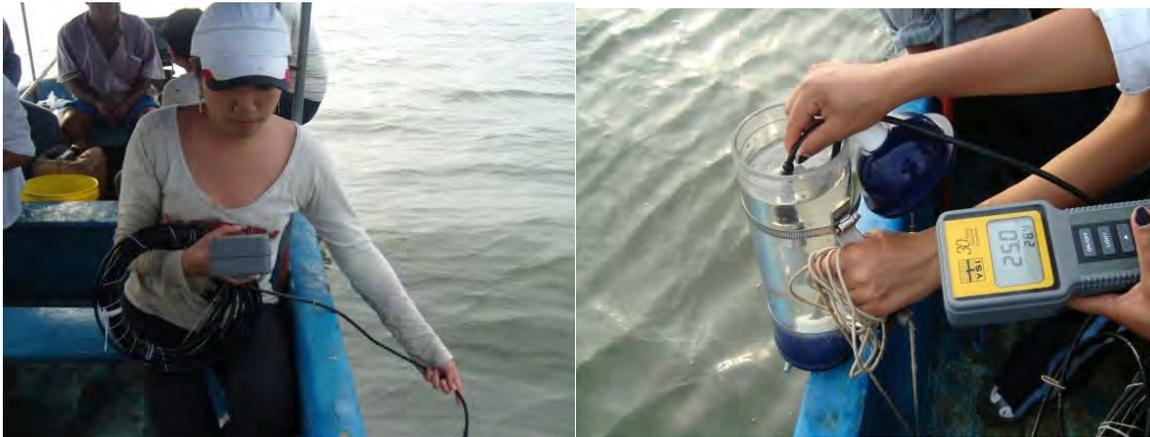
Fig.10. Multisensor YSI 30
