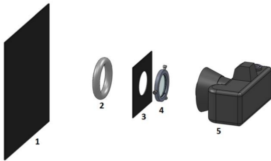
Figure. 2. Proposed illumination system for the scratch and dig measurement.
