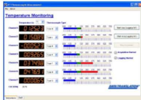
Figure 2. Use a DT9805 Series module with the free Thermocouple Measurement application for immediate linearized temperature measurements without programming. Simply connect the module to the PC using the supplied USB cable, connect your thermocouple inputs, and run the application. This view shows the temperature measurements of all 7 thermocouple inputs and the CJC channel in a digital display.
