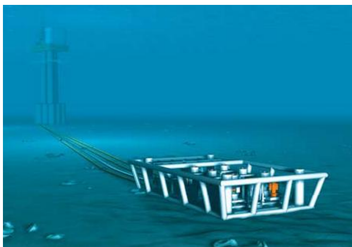
Figura 2.5 Template,(North East Frigg, Noruega, FMC Technologies).
