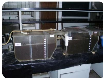
**Figura 5-1 Reactor aerobio**
