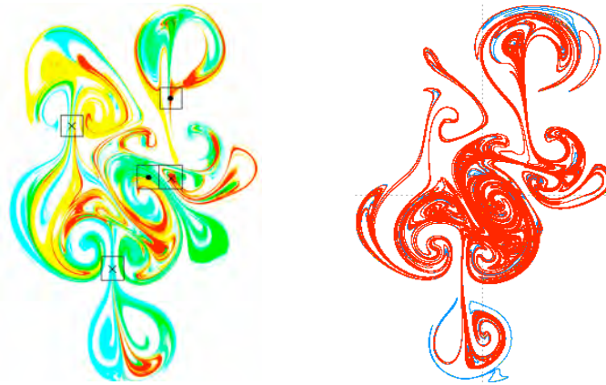
Figure 4.5: Flow due to a disordered array of five magnets at phase \varphi = 8/10 \pi . a) Experimental visualization. b) Numerical Lagrangian particles tracking. The squares denote the footprint of the magnet. The black dot ( \bullet ) and the cross ( \times ) denote a magnet with its dipole moment pointing in the positive and negative z -direction, respectively. Forcing frequency f_x=50 mHz. Phase-shift \phi_x = 0 .
