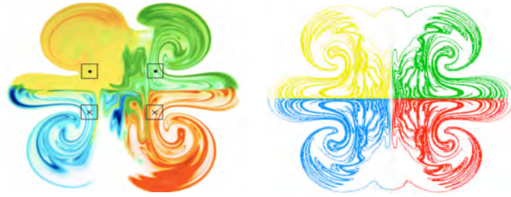
Figure 4.4: Oscillating vortex in an octopolar magnetic field at phase \varphi = 18/10 \pi . a) Experimental visualization. b) Numerical Lagrangian particles tracking. The squares denote the footprint of the magnets. The black dot ( \bullet ) and the cross ( \times ) denote a magnet with its dipole moment pointing in the positive and negative z -direction, respectively. Forcing frequency f_x=100 mHz. Phase-shift \phi_x = 0 .
