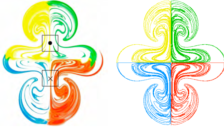
Figure 4.3: Oscillating vortex in a quadrupolar magnetic field at phase \varphi = 8/10 \pi . a) Experimental visualization. b) Numerical Lagrangian particles tracking. The squares denote the footprint of the magnets. The black dot ( \bullet ) and the cross ( \times ) denote a magnet with its dipole moment pointing in the positive and negative z -direction, respectively. Forcing frequency f_x = 100 mHz. Phase-shift \phi_x = 0 .
