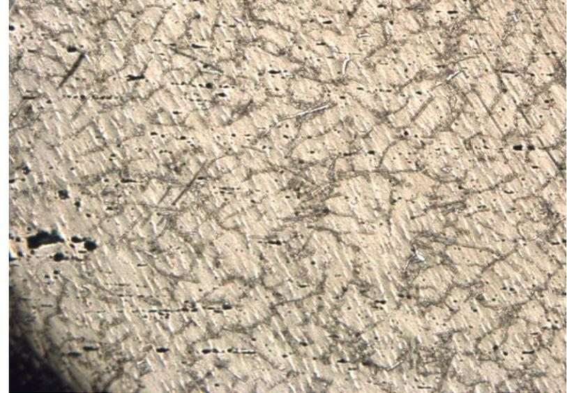
Figura C6. Al – 5.34 Si. Centro probeta **100X**.
