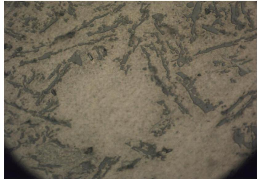
Figura C14. Al – 12.19 Si. Centro probeta **1000X**
