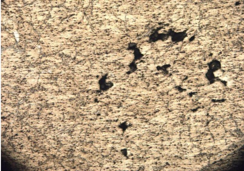
Figura C5. Al – 4.33 Si. Centro probeta **100X**.
