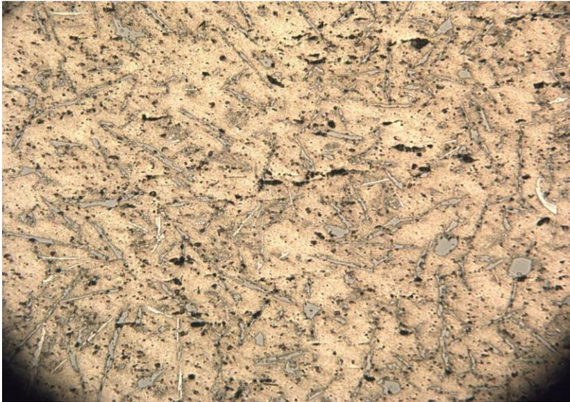
Figura C13. Al – 12.19 Si. Centro probeta **100X**
